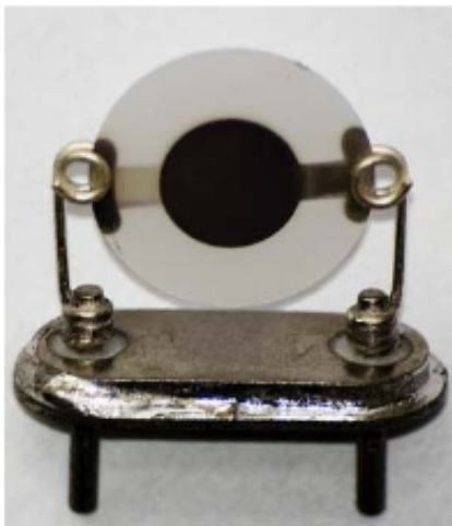
Quartz crystal plate used in electronics
