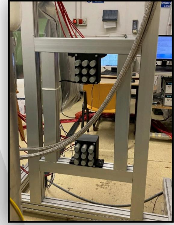
**Neutron spectrometer:** 18 Plastic Scintillators (PScis)
