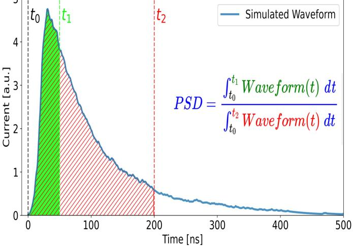
We are defining and implementing an electronic version of this concept on a custom chip (PSD ASIC) that discriminates between neutrons and gammas based on the quantity PSD, as defined above.
