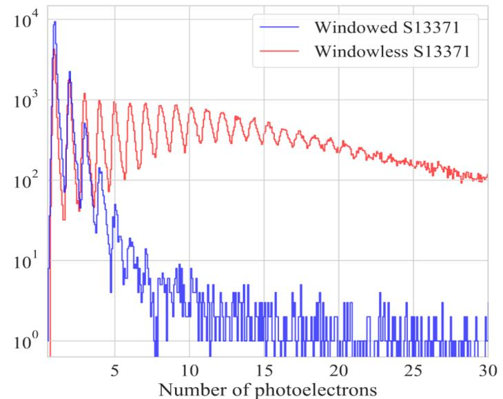
Average SiPM waveforms (left) and energy spectra measured with windowed (blue) and windowless (red) VUV SiPMs for  $^{241}\text{Am}$  radiation in pure liquid argon, confirming 128nm sensitivity
