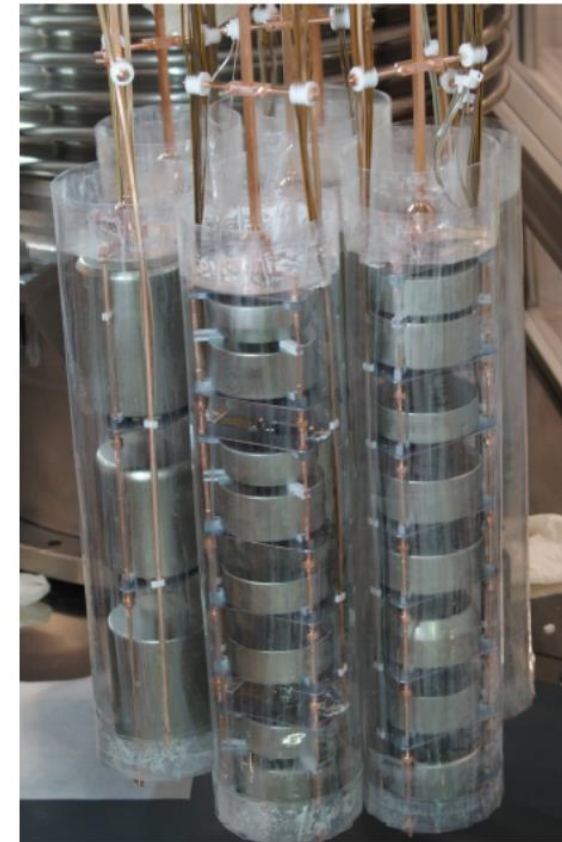
New TPB coated nylon mini- shrouds to reduce attraction of ^{42}\text{K} ions (from decays of ^{42}\text{Ar} ) to n^+ surface
