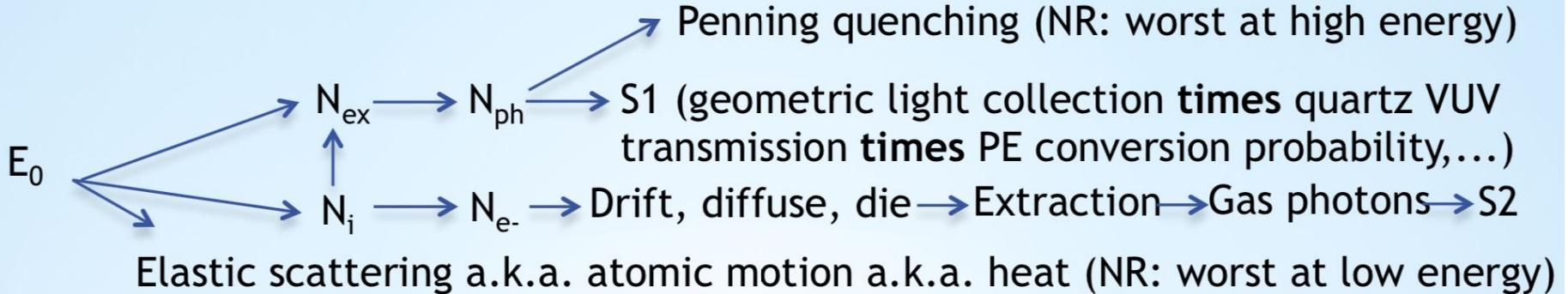
NEST started as a tool to provide a framework (usually referred as **NEST model**) to describe the process, then with global fitting of **all existing calibration data** to obtain parameters, to allow **accurate simulation** for current/future detectors.
