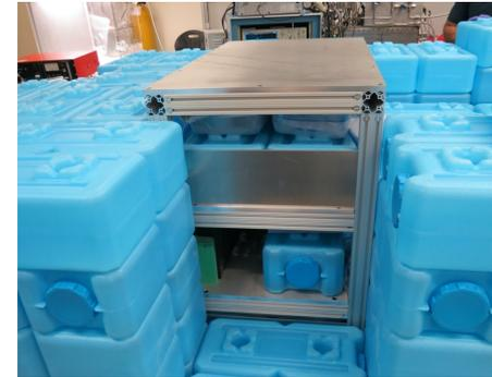
DT stand frame, constructed and partially shielded
