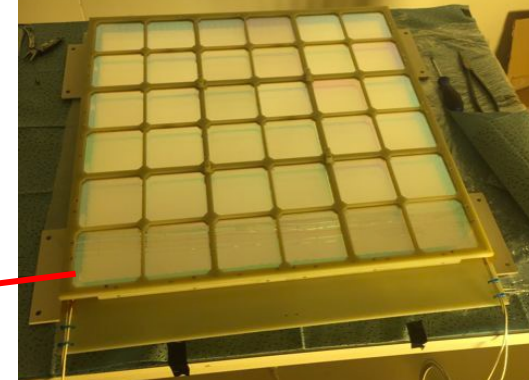
Megacell: new version of the photon detection system
