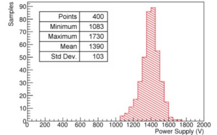
PMTs equalized  $G=10^7$  using the **Power Law** fitted from the 5 gains as function of the applied voltage.
