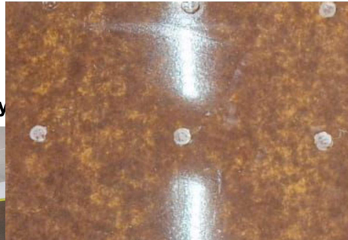
Bakelite surface roughness
