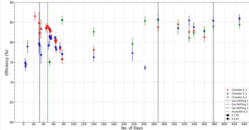
Efficiency Scan shows: Detectors are operating with **>85% efficiency**
