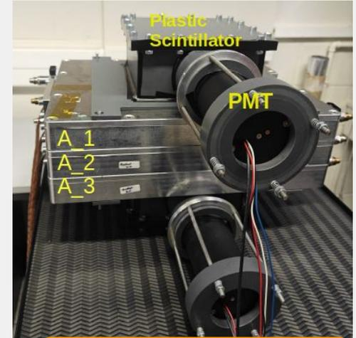
Experimental setup for efficiency measurement
