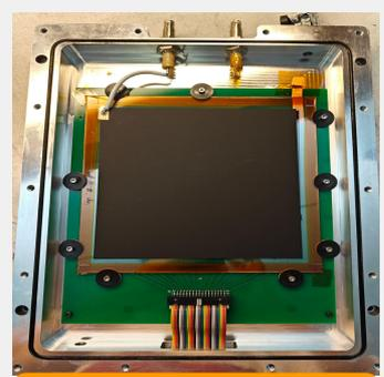
Assembled Chamber before gas filling
