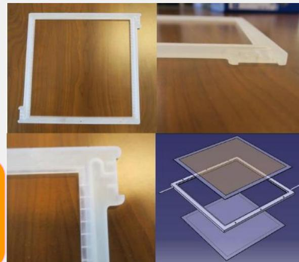
3D printed frame that requires lower gas volume only in the gas gap instead of the entire outer casing in the current version
