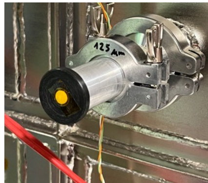
Alignment – BGO CCD gamma camera & lead plugs:
