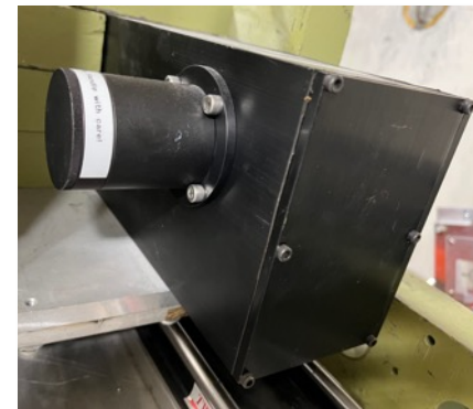
Alignment – BGO CCD gamma camera & lead plugs:
