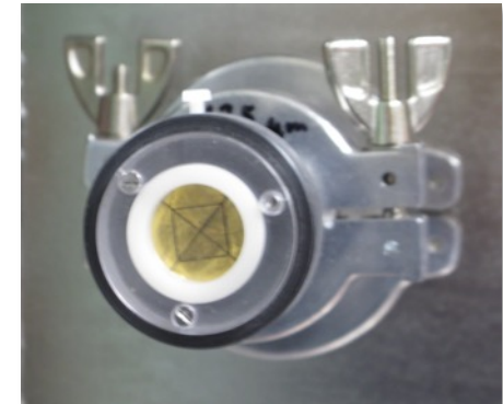
Au foil activation (downstream)
