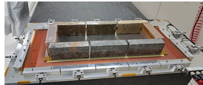
Thin glue film on the frames: “S” pattern + “void area” around the holes, to prevent glue in the holes
