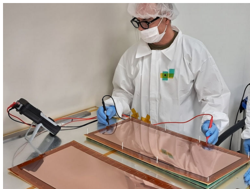
Quality control: testing the GEMs with the MEGGER
