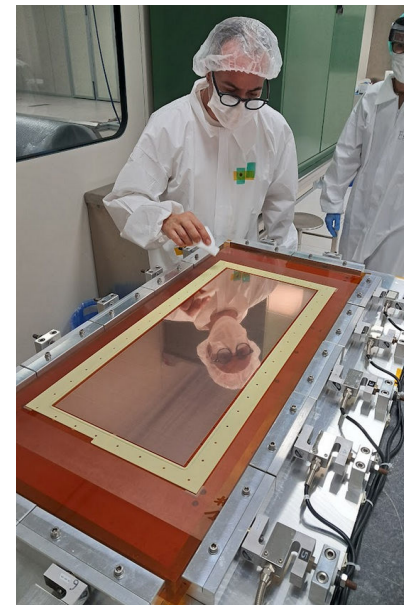
Thin glue film on the frames: “S” pattern + “void area” around the holes, to prevent glue in the holes
