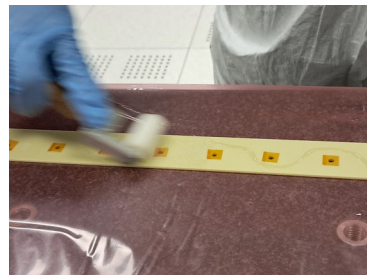
Thin glue film on the frames: “S” pattern + “void area” around the holes, to prevent glue in the holes
