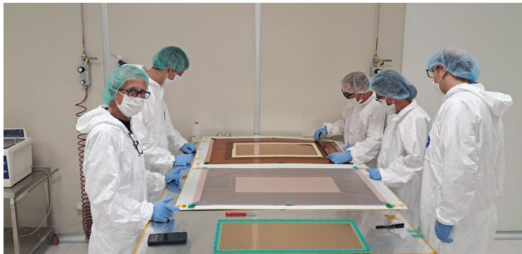
Quality control: testing the GEMs with the MEGGER
