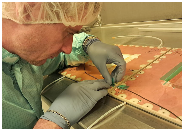
GEM 2mm frame o-ring gluing
