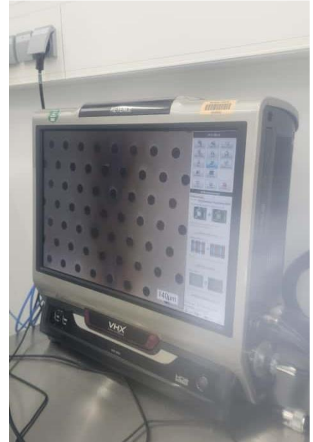
Microscope with semi-automatic analysis of e.g. hole diameter
