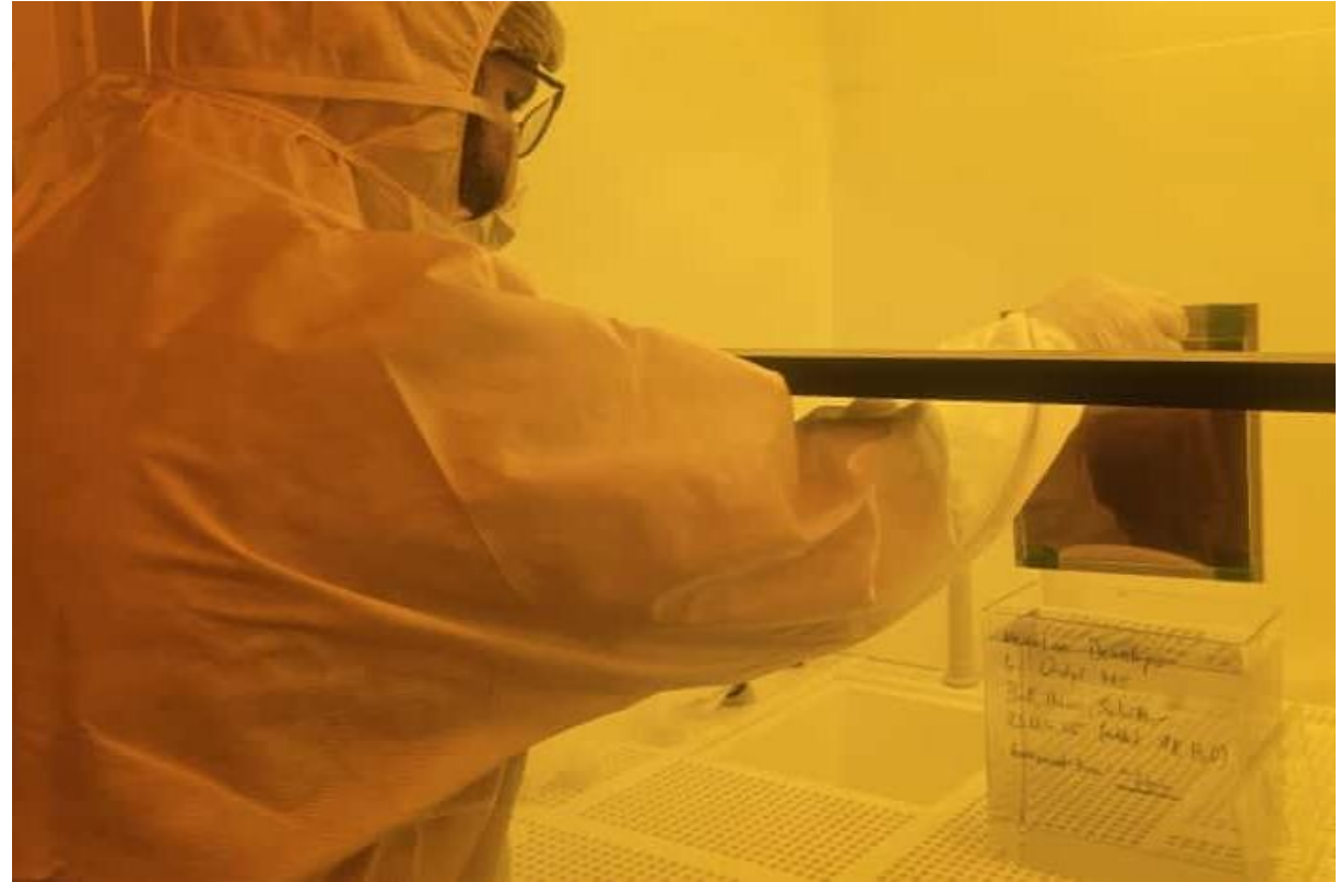
Development of the sample at the wet bench, \approx 3 min, moving the sample from time to time
