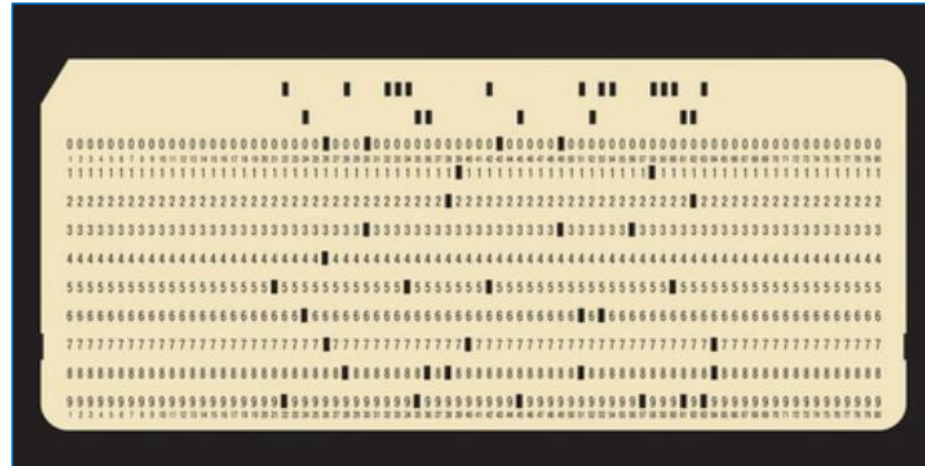
IBM 80-column, punched card
