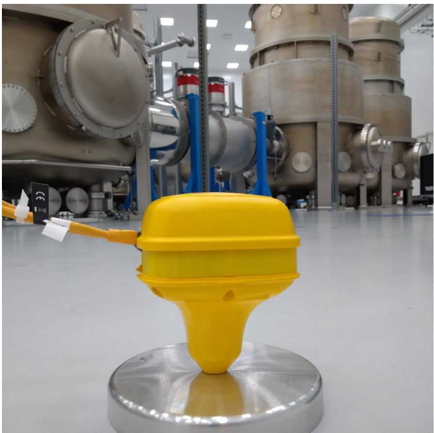
Based Innoseis seismic sensors, 4.5 Hz, geophone
