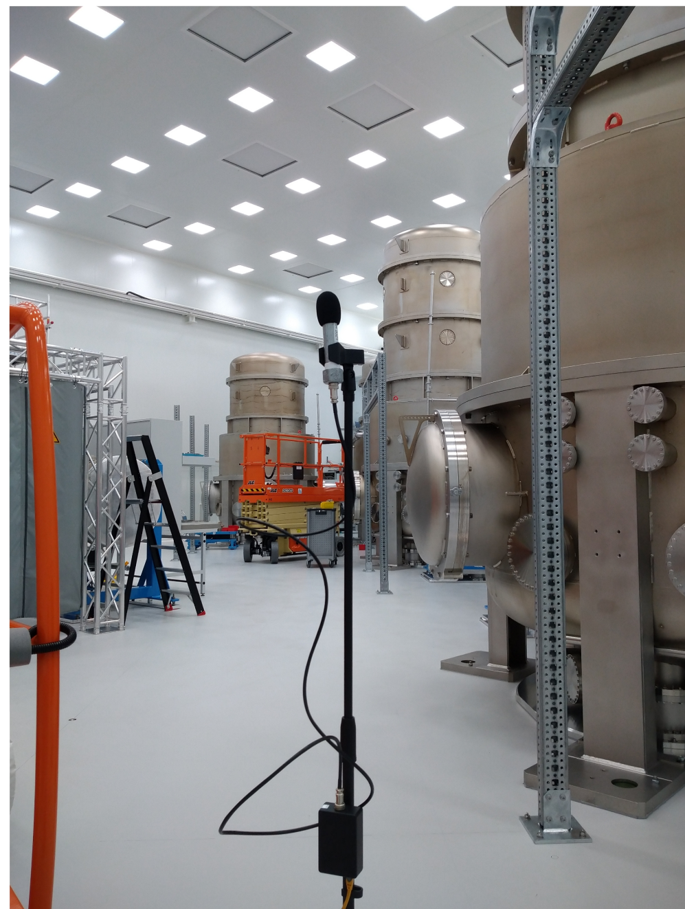
Infrasound microphone, Frequency range from 0.1 Hz to 120 Hz
