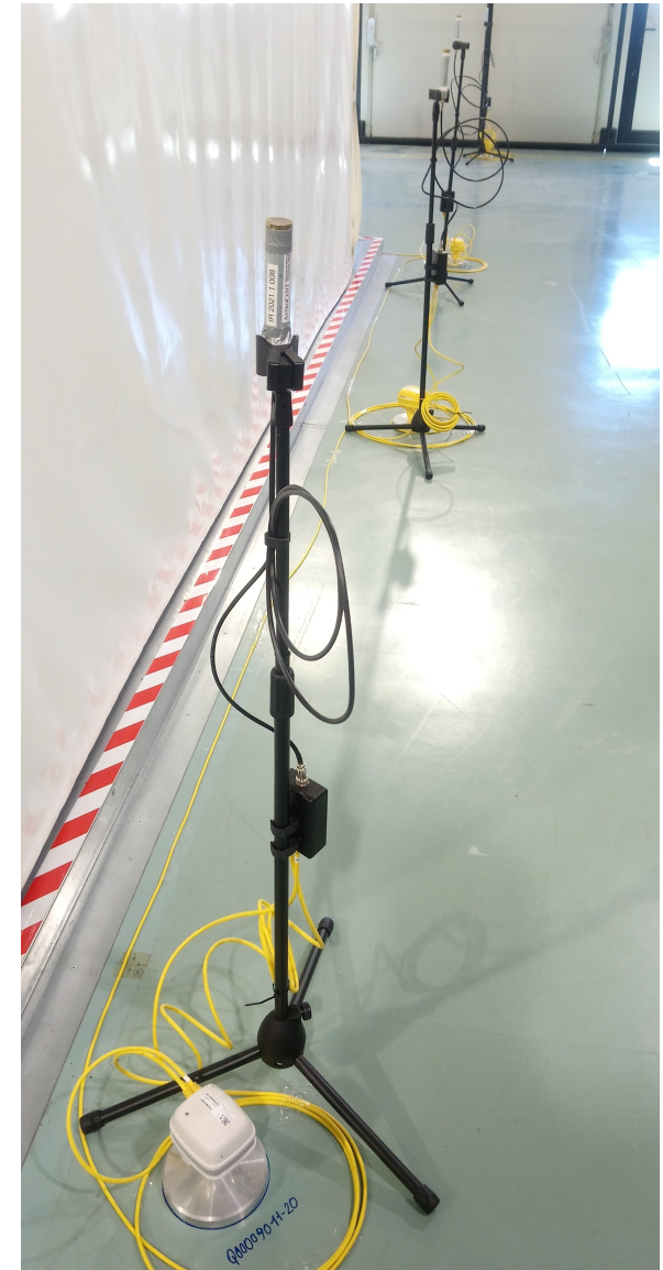
Seismic-infrasound system for Newtonian Noise cancellation in Virgo EGO.
